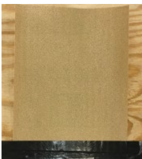
Tape sandpaper to plywood using duct tape
